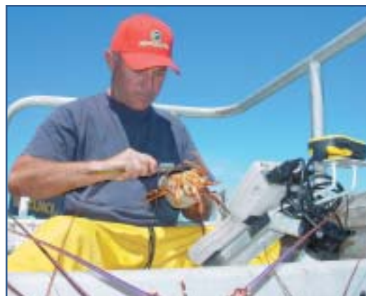
Digital calipers, GPS position, Allegro Field PC—fast, accurate recording with ERNIE. Photo credit: T. Burkhart
