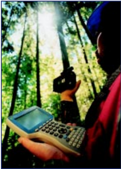
A laser rangefinder connected to an Allegro Field PC automatically records tree height.
