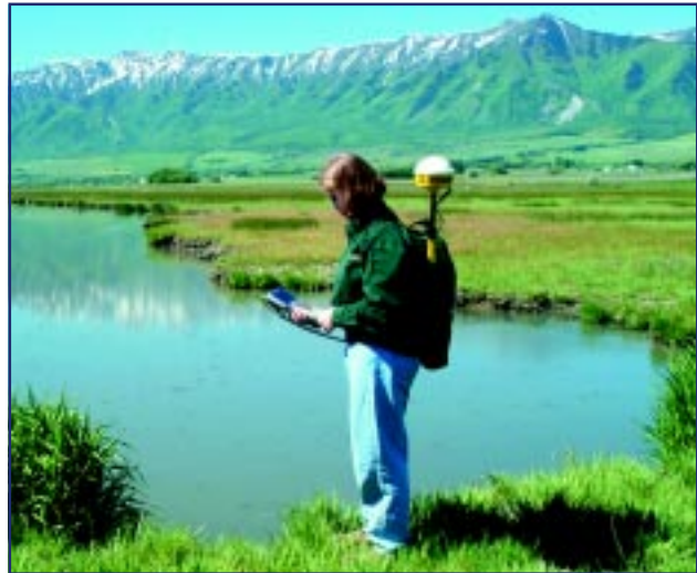
Our LandMark GPS with the Trimble AgGPS 132 receiver is used for wetland delineation to collect real-time differentially corrected GPS positions.
